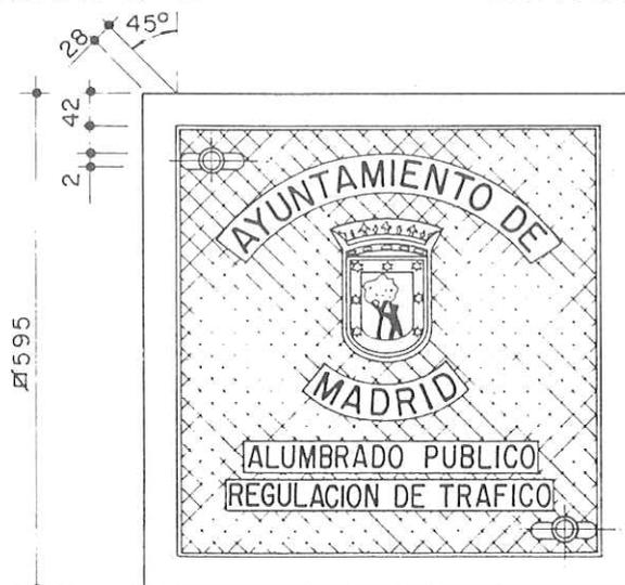
• MATERIAL TAPA: FUNDICION CON GRAFITO ESFEROIDAL TIPOS FGE 50.7 ó FGE 60.2 (UNE 3611)
