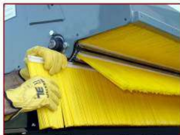
▲ Sistema rápido cambio cepillo central Fast system for changing the central brush
