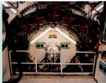
Cutterhead with installed performance of 2,800kW
