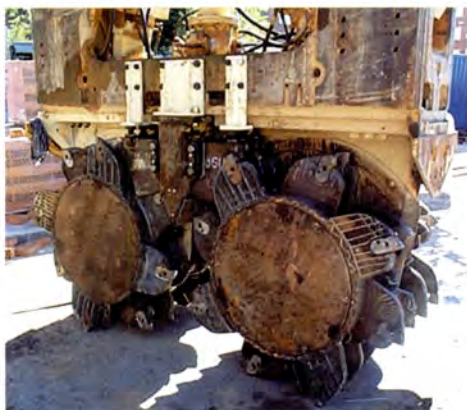
Hydrocutter used at Espartales station.
