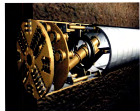
Section of EPB TBM.
