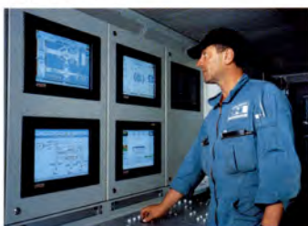
Modern TBM control panel
