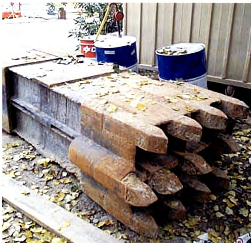
Bore bit for breaking up hard ground.
