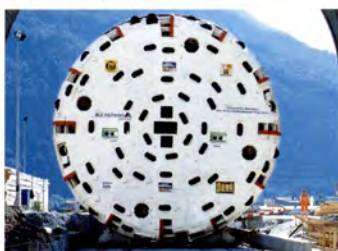
Gripper TBM, Lötschberg Base Tunnel, Section Steg Ø 9.43 m
