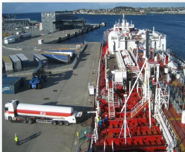
Tank truck to Ship Bunkering (TTS)
